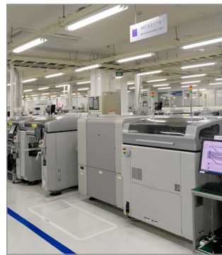
Surface Mount Technology (Chip Mounter line)
