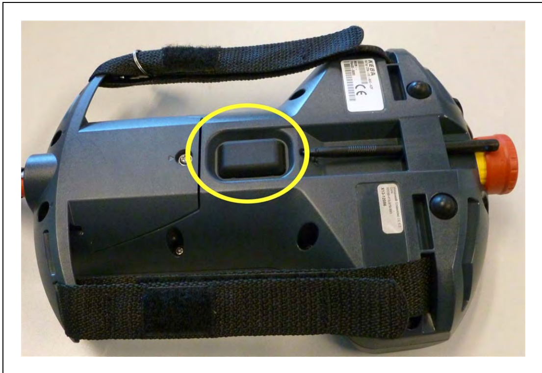
Figure 4-3. 3-Position Enable Switch (Circled)
