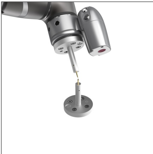
Figure 96: The Robot Posture Needs to Change during Teaching (1/2)
