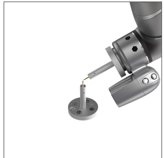
Figure 96: The Robot Posture Needs to Change during Teaching (1/2)
