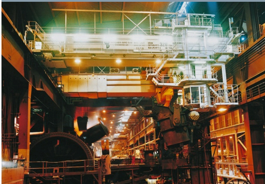
Example: Ladle crane, lifting capacity 200 - 500 t, gantry speed approx. 60 m/min
