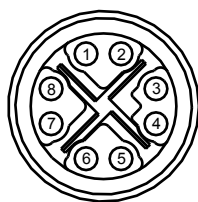
Figure 3.10 8-Pin M12 X-Coded Ethernet Port Pin Configuration
