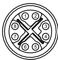
Figure 3.8 8-Pin M12 X-Coded Ethernet Port Pin Configuration
