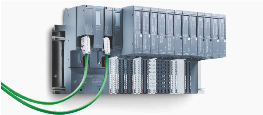
SIMATIC ET 200SP HA: Depending on the application, the distributed I/O can be operated redundantly with two interface modules or as a single station with one interface module.
