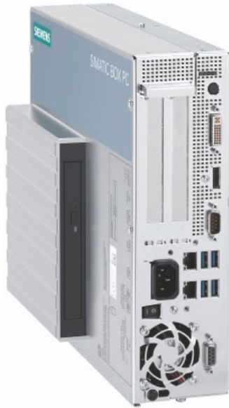
SIMATIC PCS 7 BOX RTX compact system
