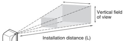
The horizontal field of view is given in the optical chart. The vertical field of view is approx. 60% of the horizontal field of view.
