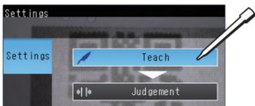
Place the object that is to be used as the measurement reference in front of the camera. Move the rectangle so that the characteristic part for position compensation is inside it.
