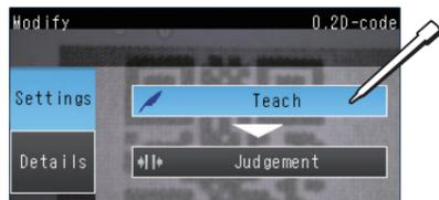
Confirm that the 2D-code is inside the green frame and touch [OK].
