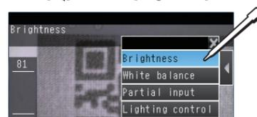
Adjust the brightness with the slider at the bottom of the display. You can also press [AUTO] to automatically set the brightness according to the image.
