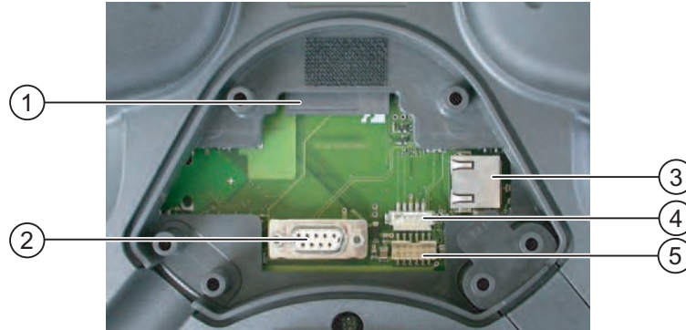
Figure 4-16 Interfaces on Mobile Panel 177 PN
